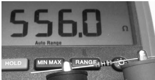
Figure 3-4: Multimeter measuring a 560-ohm 1 percent tolerance resistor
