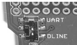
Figure 13-4: GPS shield data switch
