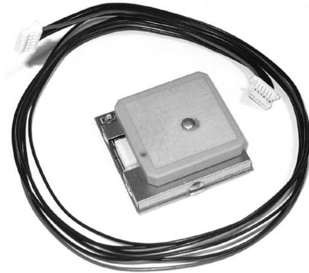
Figure 13-3: A long GPS-receiver-to-shield cable
