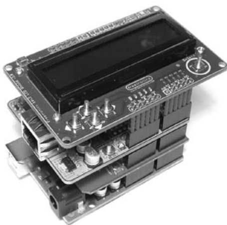
Figure 8-4: Three stacked shields with an Arduino Uno
