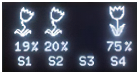
Figure 13.25 – OLED display sample of the four sensors
